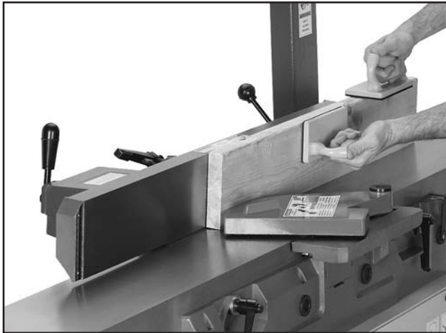
Figure 39. Example of edge jointing operation.
